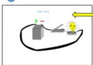
This circuit will not work because the switch is open.
